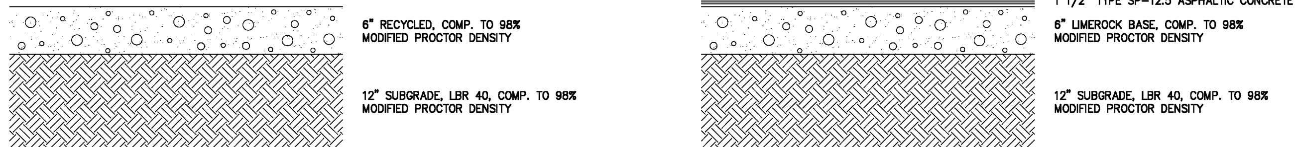
TYPICAL STABILIZED DRIVE DETAIL
